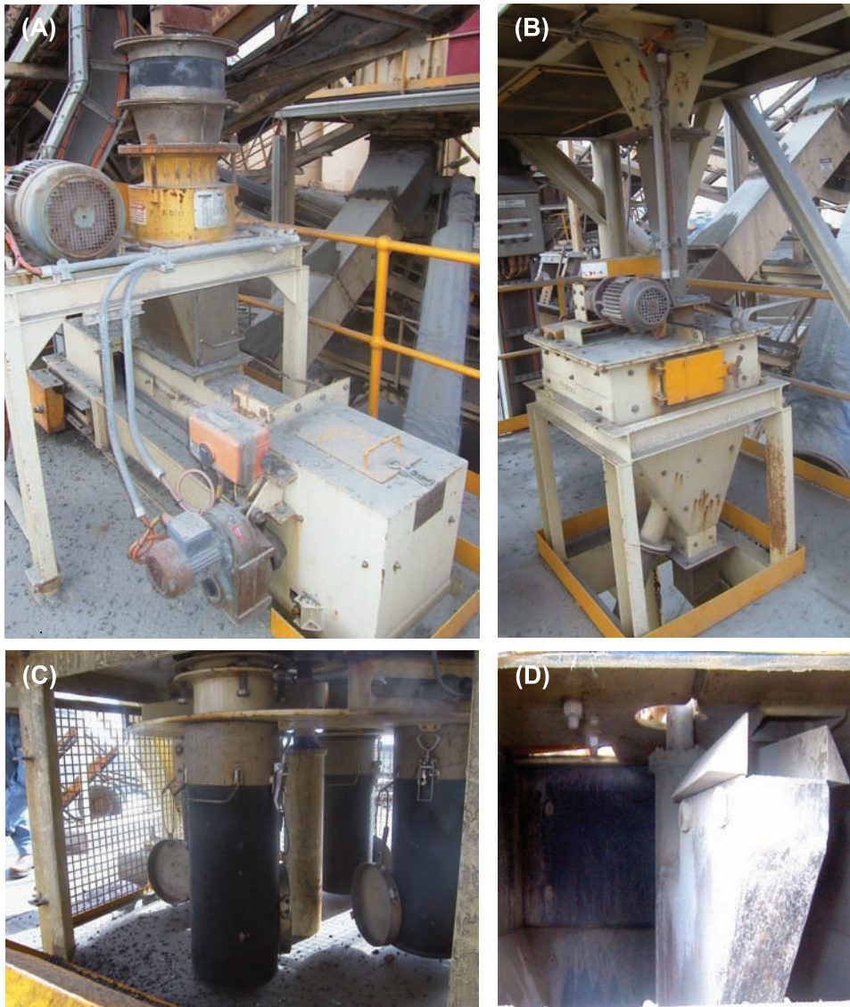
FIG 4 - (A) Sample crusher; (B) secondary sampler housing; (C) sample collection pots, and (D) secondary vezin cutter.
